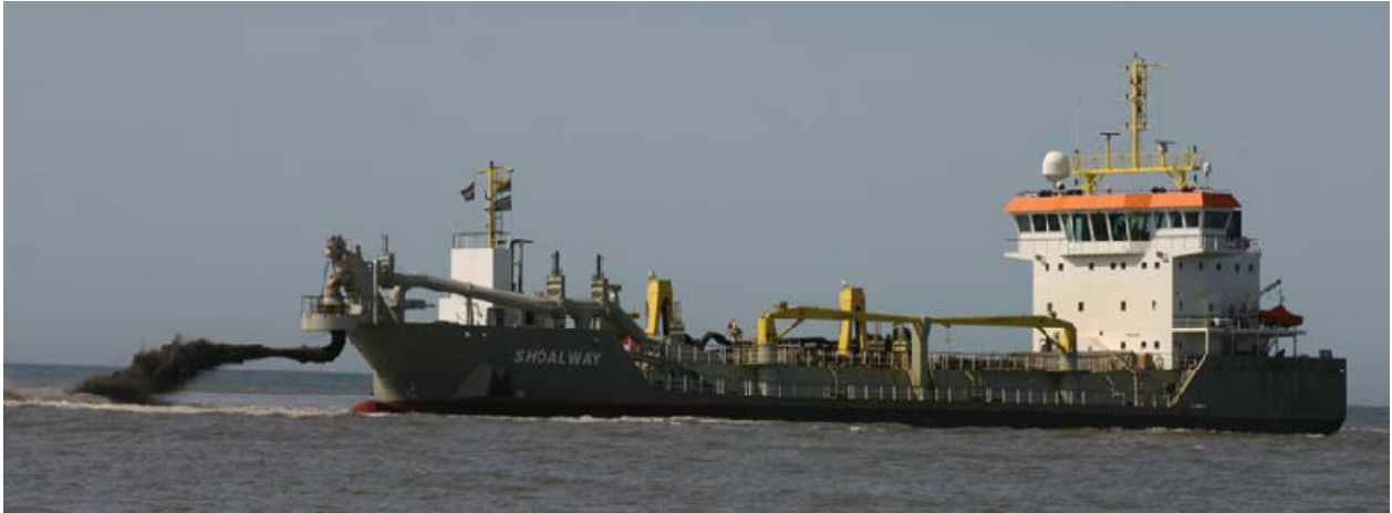
The TSHD SHOALWAY seen operating at the Zandmotor project along the Dutch coast
